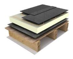
Mastergold Nordic fully bonded in a multi-layer system
